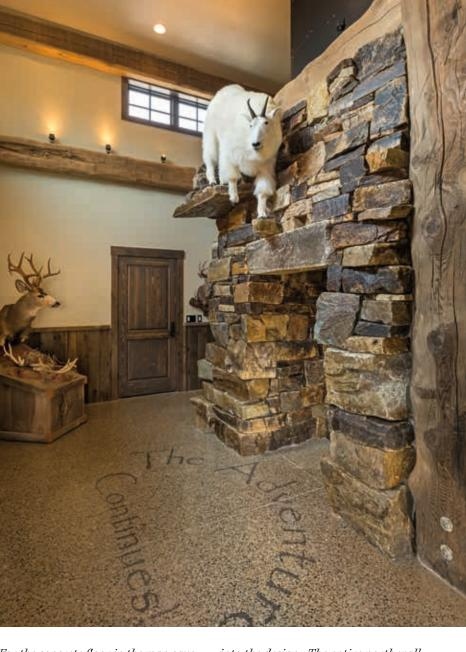
For the concrete floor in the man cave, we used an exposed aggregate mix design and used grinding company to polish it to a 3000 grit finish. In the tack room, we used a green mountain marble and "seeded" (scattered random pieces of stone onto the surface of the still wet concrete) the floor to add a splash of color. That floor was also polished to the same level of finish.
